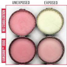
paraffin/soy Scented 70/30 candle formulation containing 0.2% stabilization in a light box with continuing exposure to black light for 72 hours.
